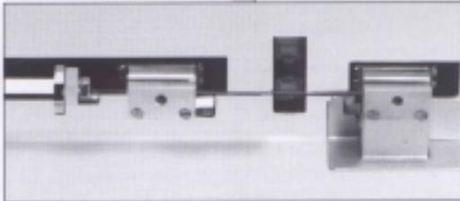
Glass tubes are clamped automatically. Fully automatic polishing of the two tips.
