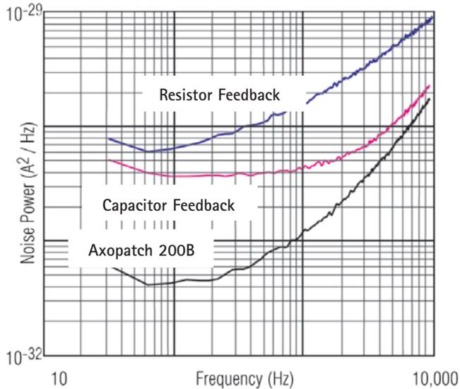
The introduction of capacitor-feedback technology significantly reduced amplifier noise (Upper trace: resistive feedback; middle trace: capacitor feedback). With active cooling, the Axopatch 200B Amplifier dramatically reduces noise to the lowest levels ever, over the entire bandwidth range (bottom trace: Axopatch 200B Amplifier).
