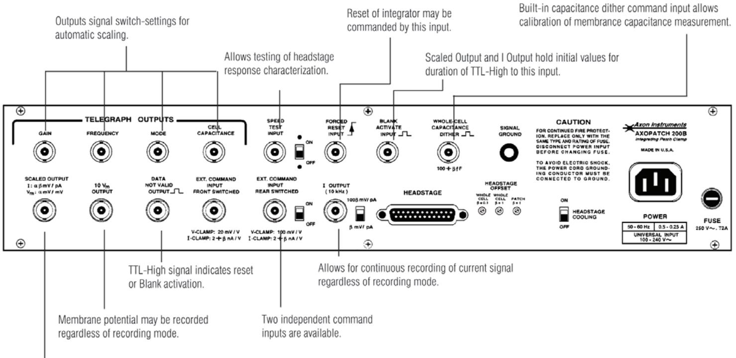
Scaled output is available from both front and rear panels.
