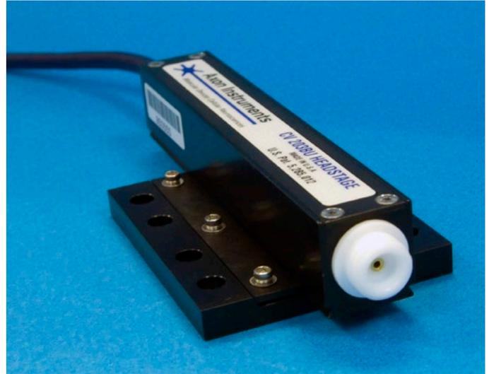
The actively cooled CV 203BU capacitor feedback headstage used for the Axopatch 200B Microelectrode Amplifier provides ultra-low noise performance in a slim package.
