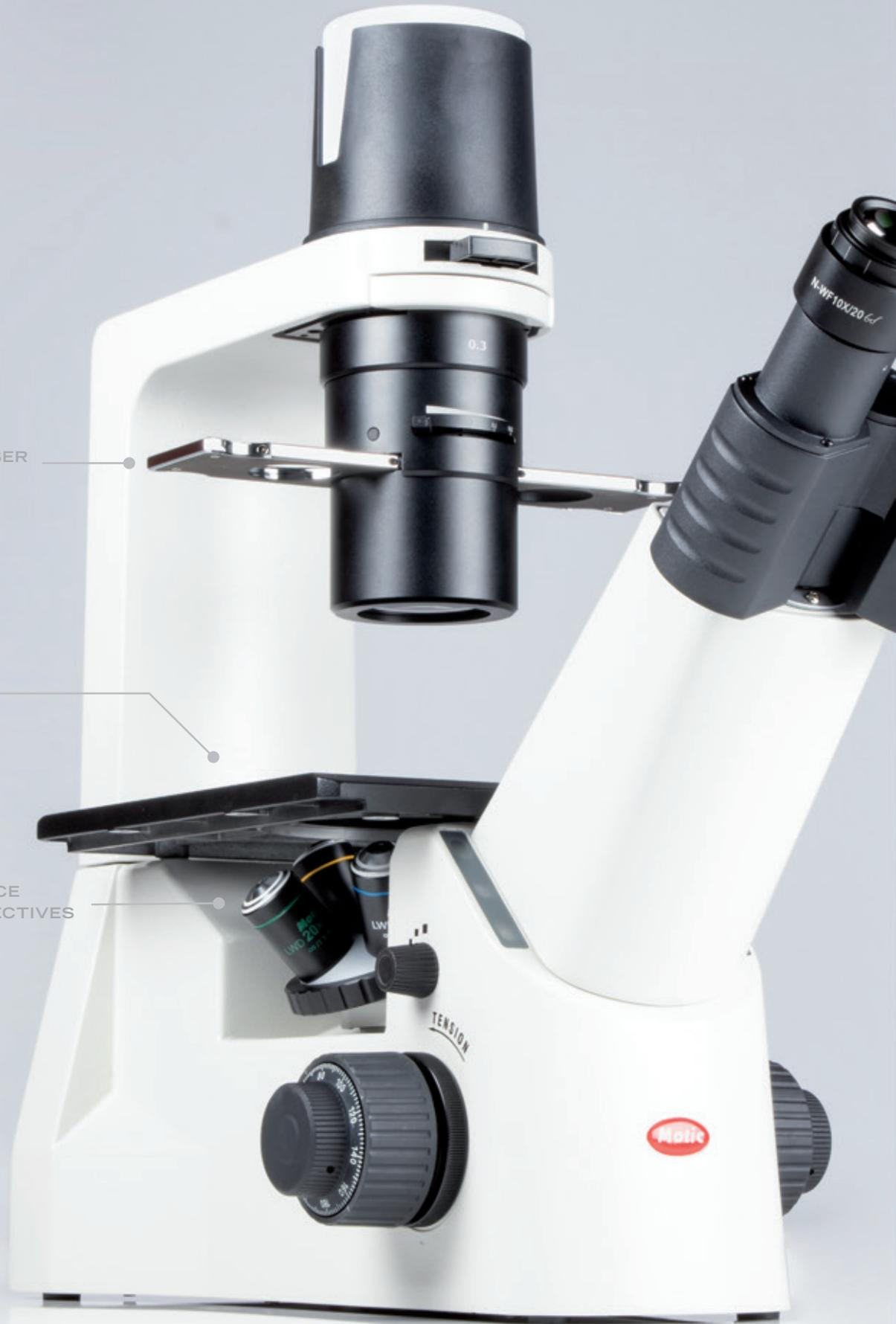
optional 4X Phase objective is dedicated to fast screening. A 40X Phase objective is available too. The AE2000 stand carries a quadruple nosepiece with a precise click stop. Rich illumination power is given by the 30W Halogen light source in a Fixed-Koehler setup, simply interchangeable with 3W LED modules of different color temperatures. The Auto ON/OFF function is a contribution to workplace safety.
