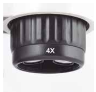
2X/4X Objective turret magnification
