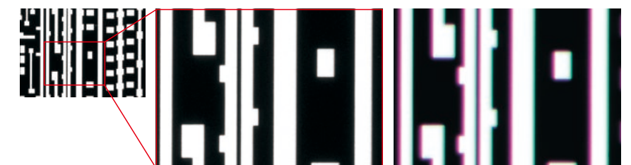
Apochromat optics (captured with SMZ1270+P-Plan Apo 1x/WF)
