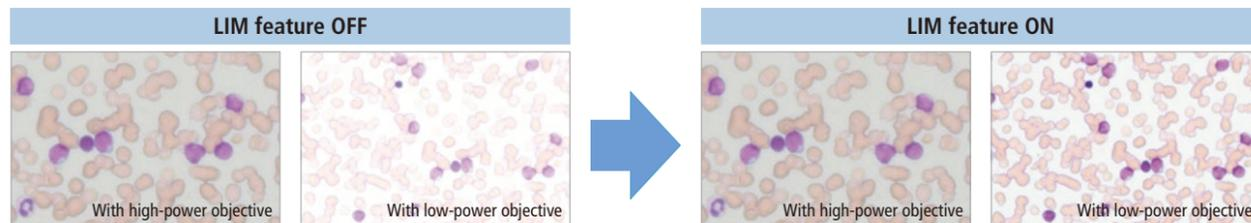
Since brightness varies depending on the objective, switching magnifications can induce eye strain.
