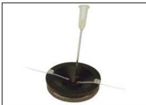
bottom up with the suction at the top of the oocyte. There is plenty of room for electrode manipulation. The chamber uses a cover glass as its bottom and a double o'ring to clamp the cover glass to the chamber.
