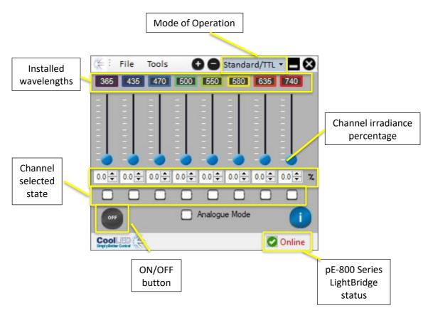
The LightBridge allows the full control of the pE-800 Series Illumination System. The above example shows the installed wavelengths of a pE-800 SB model, and these will differ if you have a pE-800 MB model or pE-800<sup>fura</sup> model. Any of the eight installed channels can be operated at the same time.
