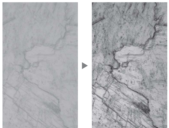
Contrast enhancement by HDR (Sample: Sliced magnesite)
