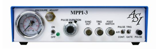
The Milli-Pulse Pressure Injector, MPPI-3 produces gas pressure pulses to an injection pipette. The unit offers precise linear control of both pressure and pulse duration. Alternatively, an external source such as a signal generator can be used to control the pulse width and rate.
