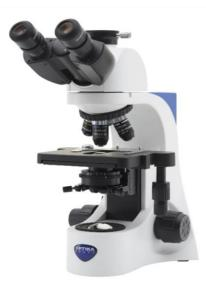
Trinocular brightfield microscope, 1000x, N-PLAN objectives
