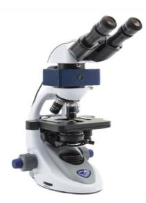
Binocular LED fluorescence microscope, 500x, IOS objectives, blue filterset
