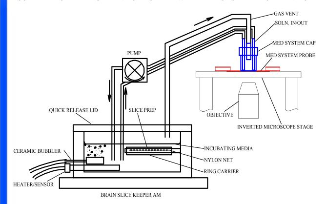
Pipes and tubes should be as short as possible and arranged to be well thermally insulated to minimise the temperature drop from the incubating area to the recoding area. The PTC03 temperature controller is electrically quiet and should not produce any interference in recordings. Peristaltic pumps may need to be grounded and shielded and kept at a distance from the recording area.
