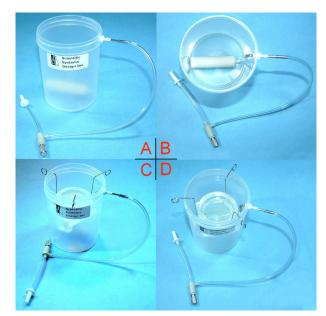
ABOVE: Components of BSK1 slice keeper and Holder BSKV: A BSKV consists of a 200ml trough fitted with a ceramic air stone and needle valve regulator for fine control of gas. B View of BSKV from above. C BSKV with BSK1 in place and D viewed from above. BELOW: Dimensions
