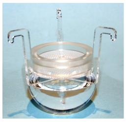
Buchner funnel with 40 to 60 micron porosity sintered glass membrane can be used instead of the BSKV. When first placing the BSK1 into the BSKV, any large air pockets are dispelled from under the net by means of a teat pipette. When in place, the fluid level is maintained at least 5mm above the upper ring of the BSK1. This ensures circulation of fluid over the top and downwards towards the slices. The typical fluid volume with BSK1 with a BSKH is 220ml and with a Buchner funnel it is 320ml.
