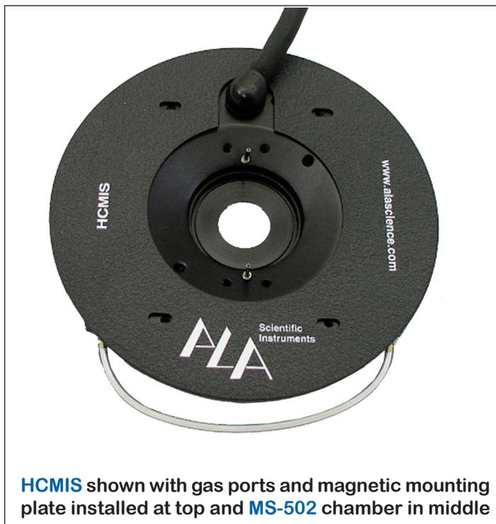
**HCMIS** shown with gas ports and magnetic mounting plate installed at top and **MS-502** chamber in middle
