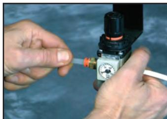
Finally, level the frame using the integrated leveling feet and bubble level indicators and plug air supply into the pre installed ARF.
