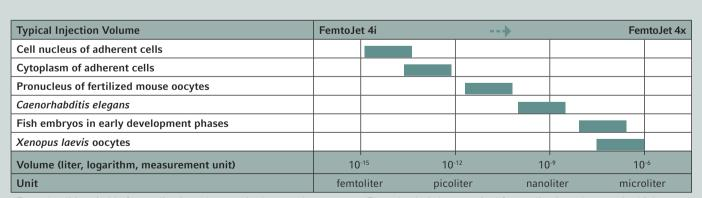
FemtoJet 4i is suitable for applications that require lower volume ranges; FemtoJet 4x is better suited for applications that require higher volume ranges. Both feature the same injection time and pressure parameters.
