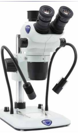
Trinocular stereomicroscope with pillar stand and ultra-flat base, illuminated stage with **X-LED**<sup>73</sup> transmitted illumination and **X-LED**<sup>3</sup> incident double arm light for outstanding brightness, freely settable.
