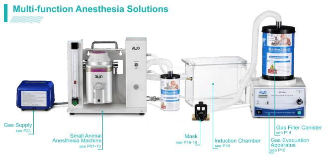
The experimental system is equipped with a gas recovery system to provide a safe experimental environment to maximize the protection of the operator; by replacing different types of anesthesia machines and masks to meet the needs of animal experiments, such as cerebral ischemia and myocardial ischemia model, osteoporosis model, tail vein injection, abdominal aorta blood sampling, heart blood sampling, ventricular injection, tissue / organ removal and other animal surgery experiments.
