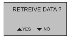
Use the UP/DOWN buttons on the front panel to select YES or NO. On the first time powering up the HCT-10 there is no data stored other than the default values.
