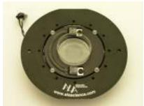
The HCT-10 parameters are set to Heat only and it is recommended to use the maximum voltage (12V) in the *OUT* setting.
