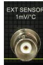
To activate this mode, use the UP/DOWN buttons to select *EX*. Connect your external monitor to the front panel BNC labeled *EXT SENSOR*.
