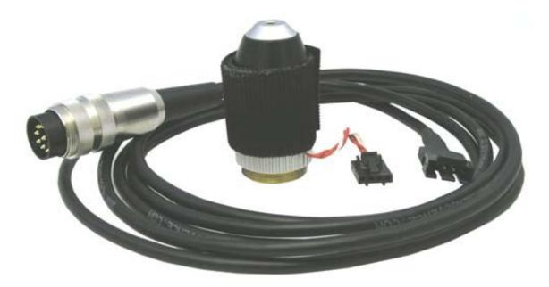
For active temperature control, the Objective heater comes with a built-in sensor that can be connected to your temperature controller. If using an npi temperature controller, an optional cable is available to connect the objective heater to the circular DIN connector on the front panel. Measure the temperature and adjust the controller as necessary. If you want, you can switch to the active control mode, and control the temperature of the foil automatically to a set temperature.
