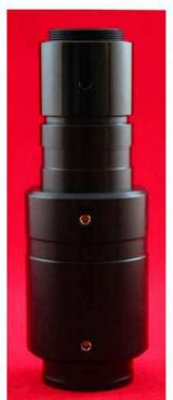
The C-Mount adapter (shown on right) would interface to your microscope - this would then supply a base for a bottom clamp, to which the optical camera adapter would then drop into, making it stable - much like the example to the left.
