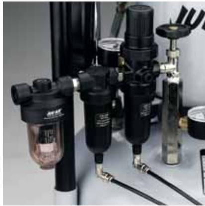
*Filters mounted on a compressor*
