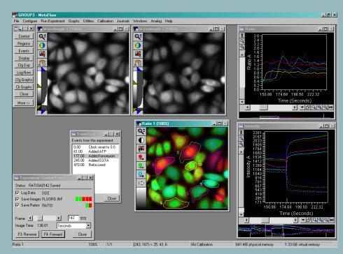
A simultaneous display of multiple wavelengths images and various customizable graphs provide an easy point-and-click interface. When playing back an experiment, clicking on the graph will rewind or fast-forward the experiment to show the images that correspond to that location on the graph.
